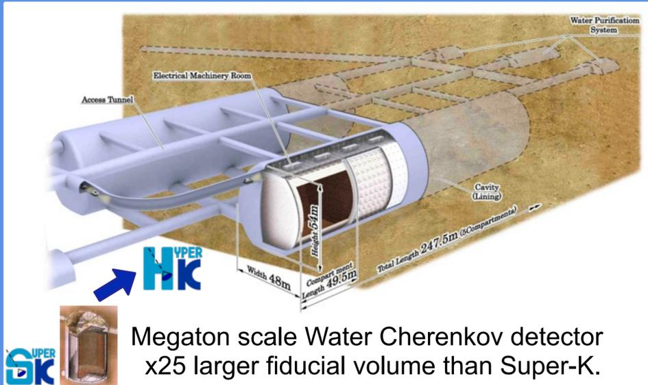
Megaton scale Water Cherenkov detector x25 larger fiducial volume than Super-K.
